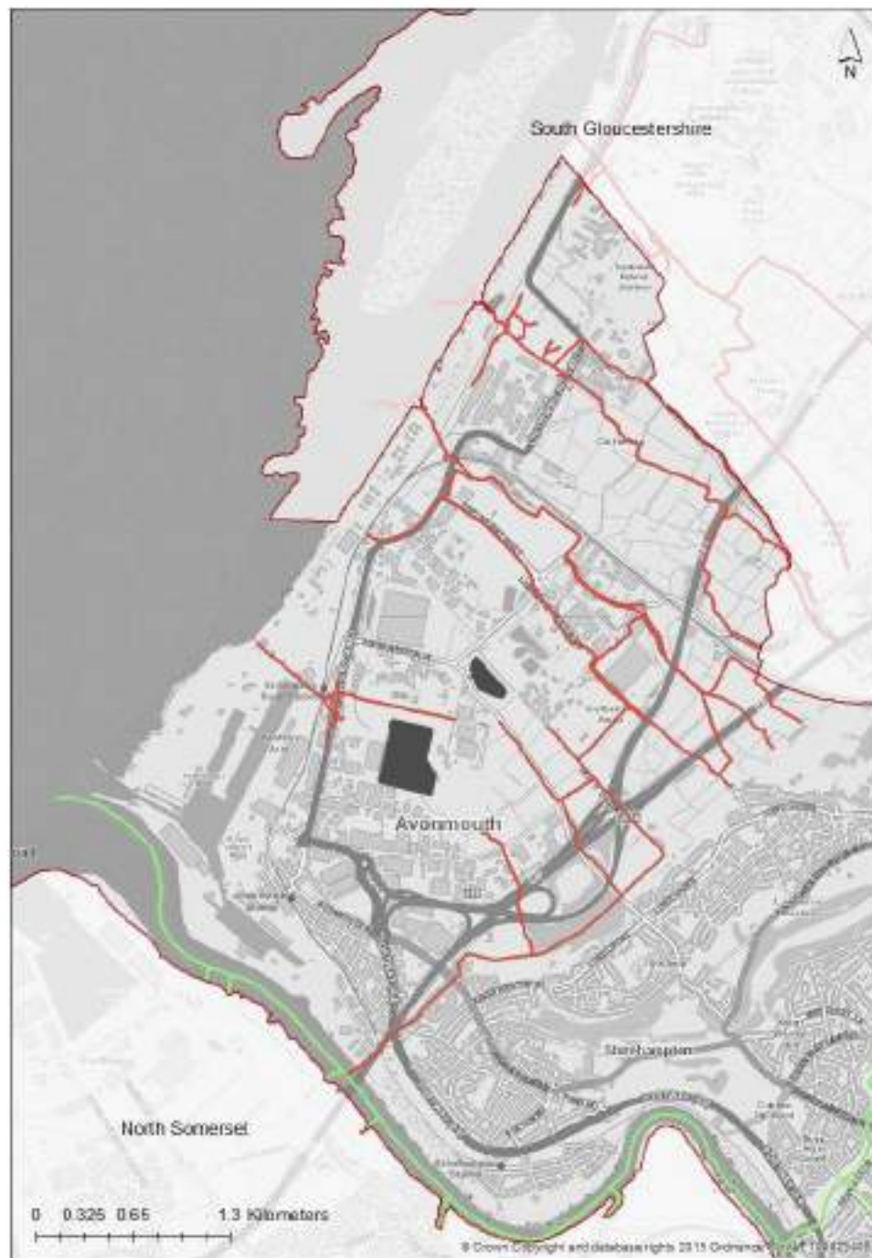
Figure 108 - Showing the significant drainage network of the Avonmouth rhine network (in red) and where it discharges into the River Avon (in green).
