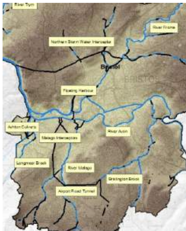
Figure 120 - Showing the open channel watercourses (in blue) and where they have been diverted by man-made, culverted, piped systems (in black) in Bristol.
