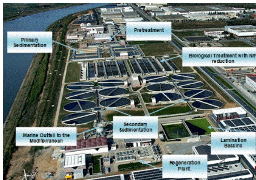
Figure 86: Current conventional treatment scheme of “El Prat” WWTP.
