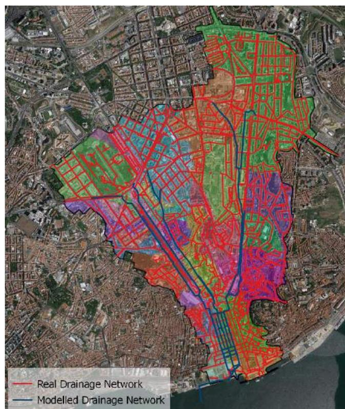
Figure 69: Real and Modelled Drainage Networks for J&L catchment.
