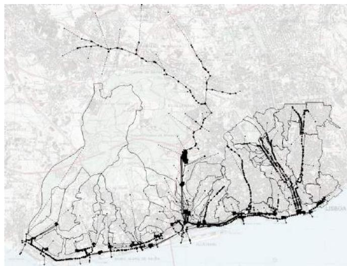
Figure 68: Modelled Alcântara Drainage System (1D SWMM Model).
